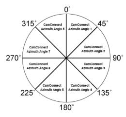
If the forbidden area is enabled on the Sennheiser Control Cockpit software, the corresponding position of CamConnect will also be affected. Example: If the forbidden area is set to 0° to 60°, the audio signal from 0° to 45° of CamConnect Array Azimuth 1 and 45° to 60° of Array Azimuth 2 will be ignored.
