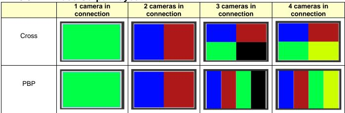
If there are three connected cameras, they will be displayed in a 4-grid layout, with one grid showing a black screen.
